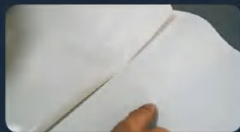
Peeling Test After Hot-welding of PVC Materials
